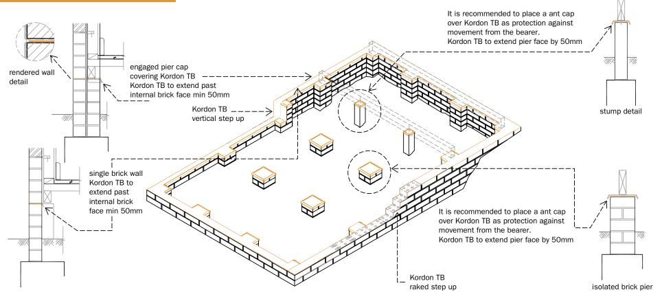
Note – Typically Kordon TB level should be a minium of 75mm clear from finished ground, or paving level. (with the exception of disabled ramps, and paved entry ways.) Sub floor clearance should be 450mm, for access of annual inspections.
